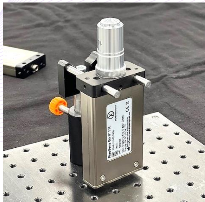
Figure 1: FluoSens Go with a 100x microscope objective lens replacing the traditional lens displayed in the background Go.
